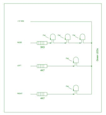
Connect +12Volts to the top of the LEDs, and to light each LED(s) pull the resistor(s) to GND
